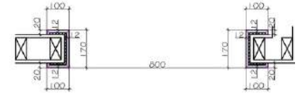
WC DOOR LINING & SETTING OUT
